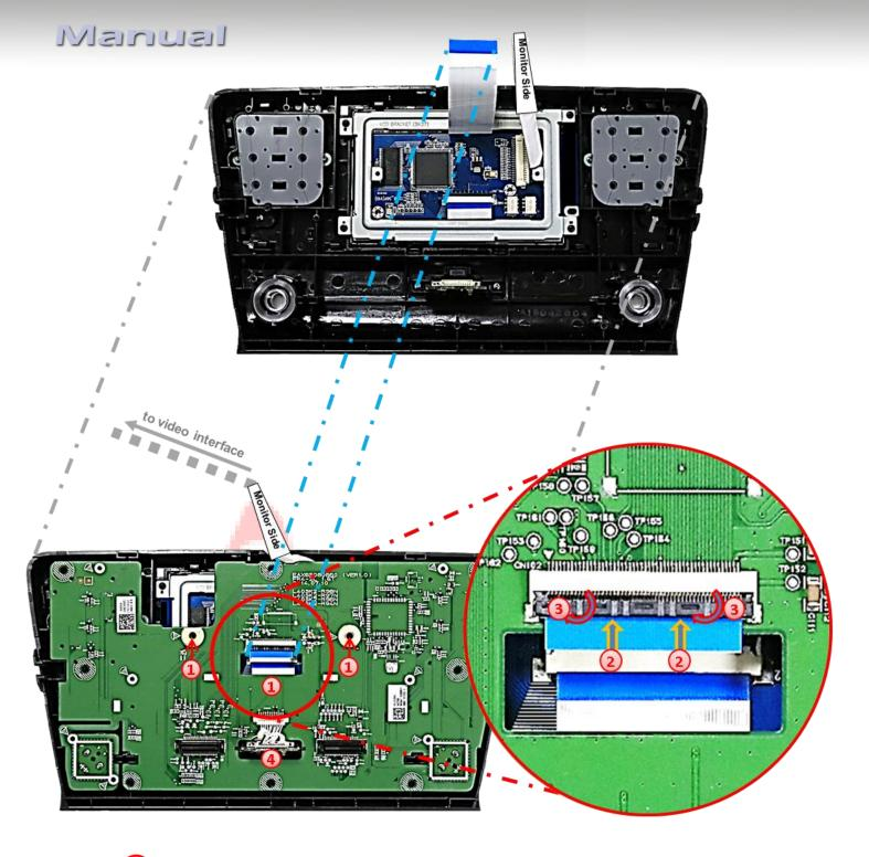
Hold the factory mainboard in its right position, lead the daughter PCB's 50pin ribbon cable **"CAR-IN"** through its recess and again, fix the mainboard with two screws.
