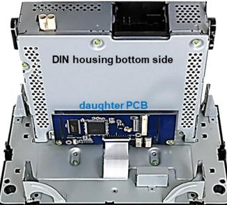
Internal PCB installation
