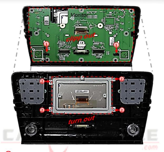
Clipp out the monitor's mainboard from the monitor's front housing and put it aside for setting free the monitor panel's metal frame and the 50pin ribbon cable for its connection to the daughter PCB.
