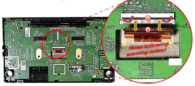
Fold upwards the black hinge of the factory ribbon cable base to unlock the original brown colored 50pin ribbon cable of the factory PCB.
