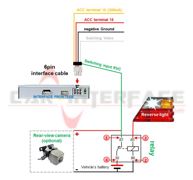
D Connect the green switching input cable to the output connector (87) of the relay.
