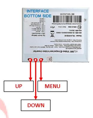
The picture settings are adjustable by the 3 push-buttons on the video-interface. Press the MENU button to open the OSD settings menu or to switch to the next menu item. Press UP and DOWN to change the selected value. The buttons are placed inside in the housing to avoid accidental changes during or after the installation. Picture settings must be done separately for AV1, AV2 and CAM while the corresponding input is selected and visible on the monitor.
