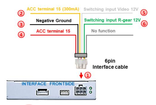
Connect the white female 6pin connector of the 6pin interface cable to the male 6pin connector of the video interface.
