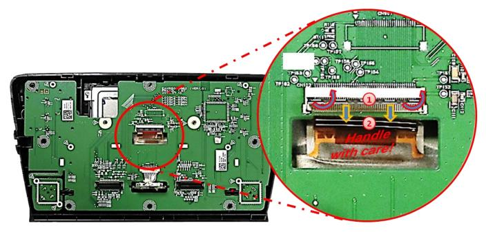
Fold upwards the black hinge of the factory ribbon cable base to unlock the original brown colored 50p in ribbon cable of the factory PCB.
