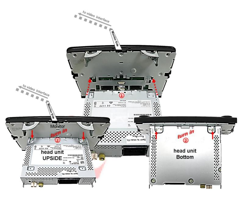
Reassemble the head unit housing to the monitor housing. Take special care for the perfect fitting of both parts and for not to get caught the small white cables of the 12pin connector.
