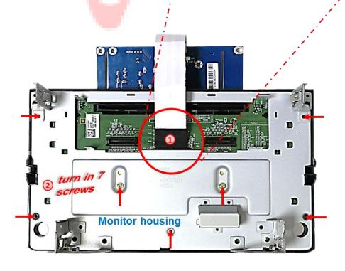
Fix the monitor's rear metal sheet by using the 7 screws.
