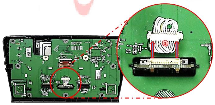
Obsconnect the female 12pin connector from its 12pin SD card connector (keep connected at mainboard).
