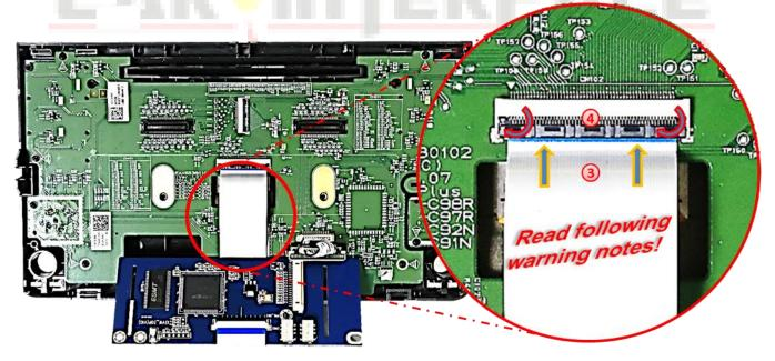
Connect the daughter PCB's 50pin ribbon cable "CAR-IN" to the previously become free 50pin ribbon cable base of the factory PCB. Make sure that the connector pins are faced to the platinum.
