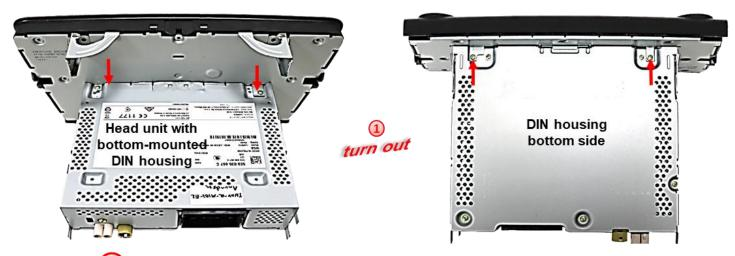
Turn out both screws at the **outer** side of the top part of the head unit (red arrows) and both screws at the bottom part of the head unit (red arrows). Separate the head unit from the monitor and lay it aside.
