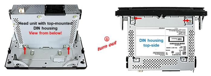
Turn out both screws at the **outer** side of the top part of the head unit (red arrows) and both screws at the bottom part of the head unit (red arrows). Remove the head unit from the monitor and lay it aside.
