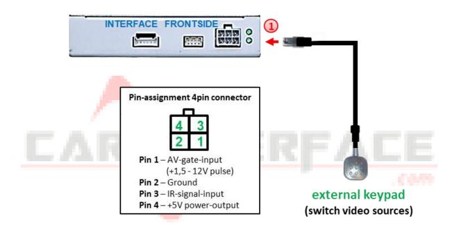
Connect the 4pin female connector of the external keypad to the male 4pin connector of the video interface.
