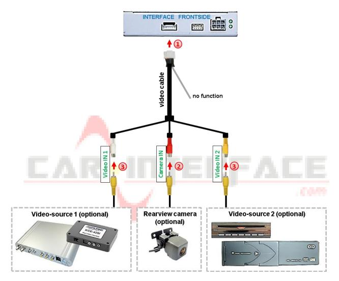
Connect the video cable's female 6pin connector to the video interface's male 6pin connector.
