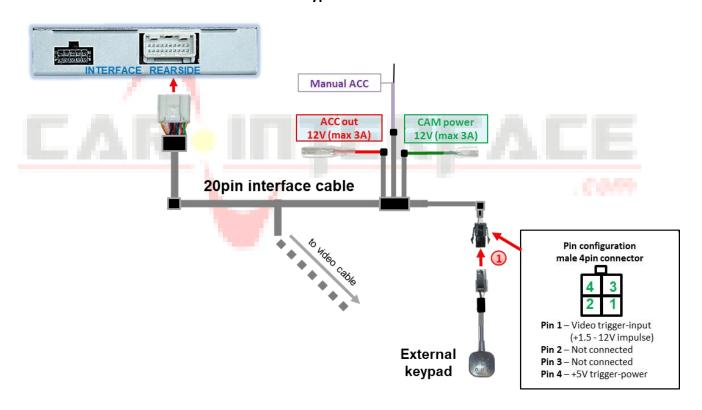
1 Connect female 4pin connector of keypad to male 4pin connector of 20pin interface cable.
