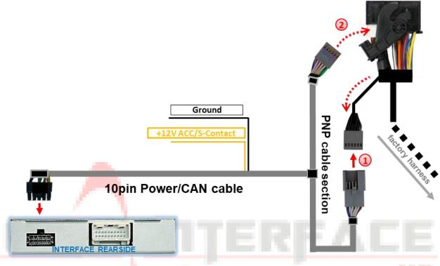
Remove the female Quadlock connector of the vehicle harness from the rear-side of the headunit and connect the previously clipped out black female 12pin connector (see graphic) to the male 12pin connector of the
