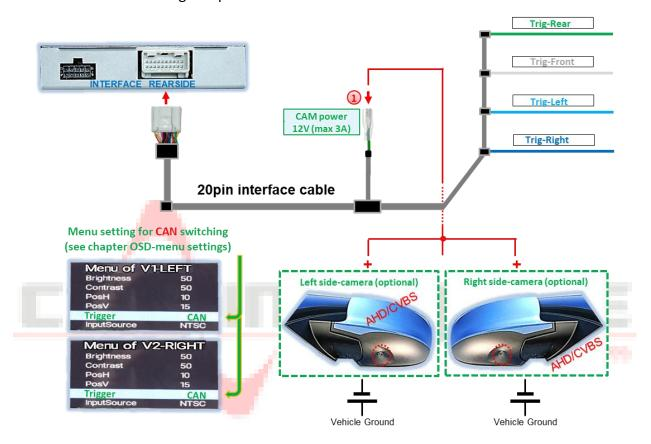
Power supply for side-cameras should be connected to green wire CAM power 12V (max 3A) of 20pin interface cable, as this cable is only powered during camera activation (some cameras are not continuously current stable).
