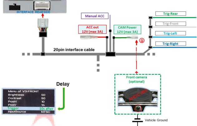
The green wire CAM power 12V (max 3A) can be used to supply power to front camera (and all other cameras connected to the video inputs), as it only carries current for the duration of any camera activation (some cameras are not continuously current-stable). Requirement is dip 3 = ON (black 8dip switch bench). Then green wire carries +12V (max 3A) as power supply for the front camera as long as the front camera input is displayed.
