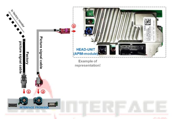
1 Disconnect the female HSD+2 connector (colours may vary) of the factory picture signal cable at the rear-side of the head unit (APIM module) and connect it to the waterblue male HSD connector "TO LCD" of the interface.
