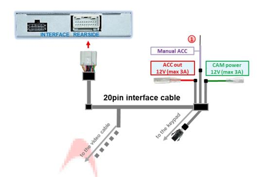
1 Connect purple wire Manual ACC of 20pin interface cable to +12V S-contact terminal 86s or ACC terminal 15r of vehicle (e.g., cigarette lighter, glove compartment illumination).
