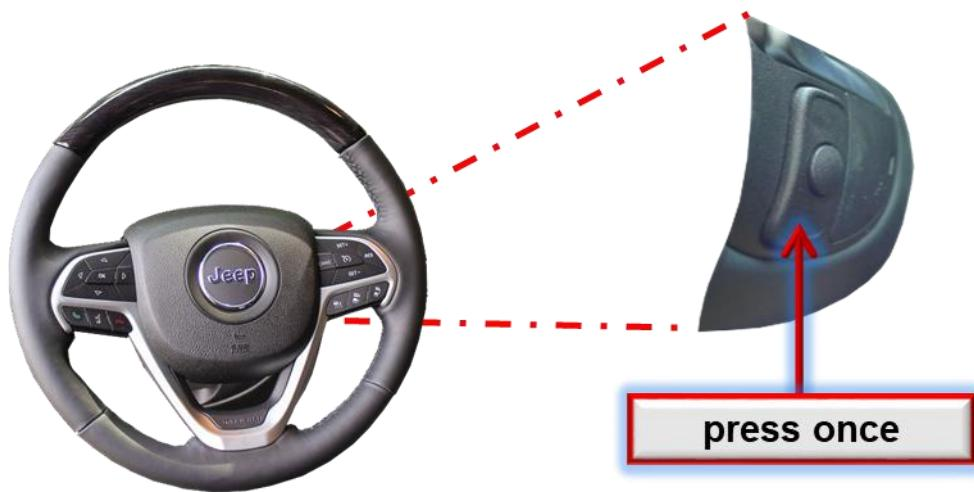
The volume button on the right-hand side of the steering wheel can be used to switch between activated video sources on the interface. If all inputs are activated via the dip switch setting, the order is as follows:
