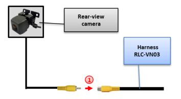
Connect the video RCA of the after-market rear-view camera to female RCA connector of harness RLC-VN03.
